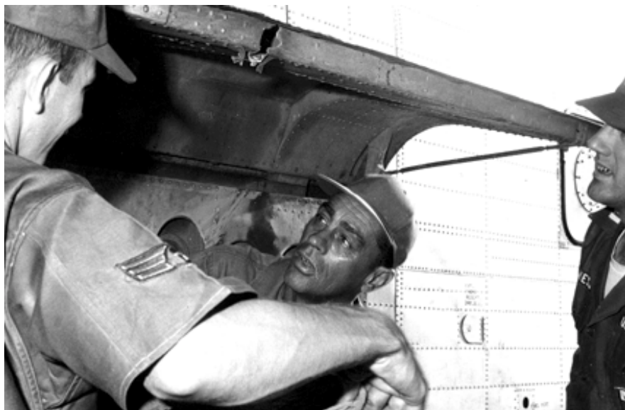
MSgt. James C. Kafferly (center), a flight line supervisor, inspects a Ranch Hand aircraft for damage, in this case a hole ripped open by a .50-caliber bullet.
